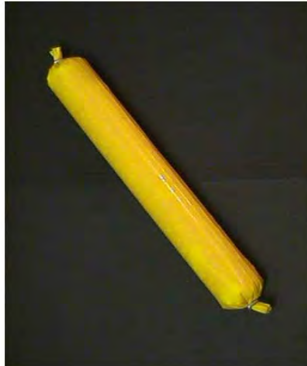
Slurry/gel mixture TOVEX is one brand name
